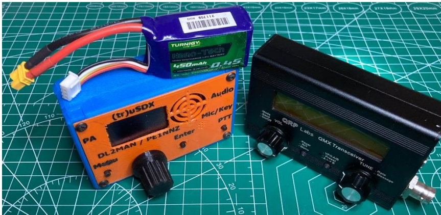
← QRP transceiver shoot-out: (tr)uSDX vs QRP Labs QMX. 3 cell LiPo battery for scale.
