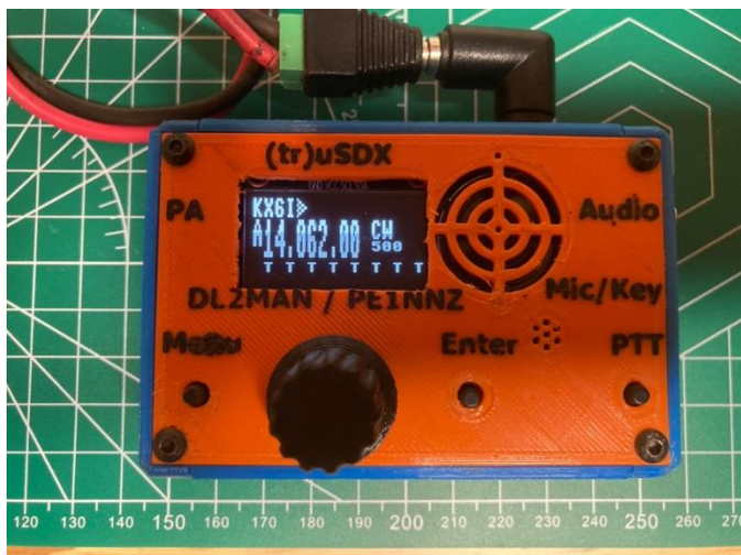
← Note that this (tr)uSDX has been modified with a larger OLED screen and tweaked for maximum brightness.
